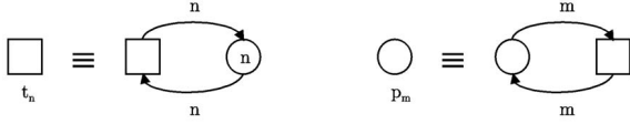
Fig. 4. Subnets of a sort n of a transition t and a sort m of a place p .
